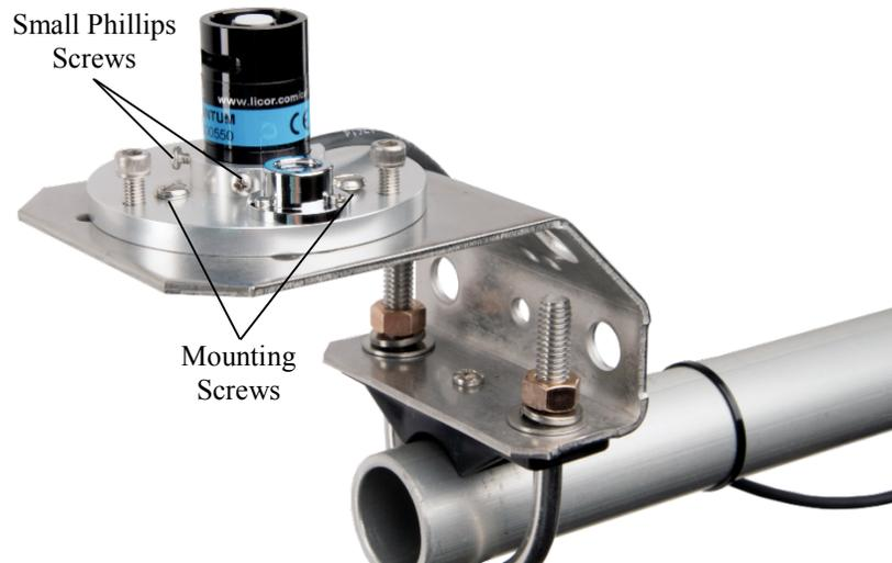
4. Loosely mount the LI2003S base/leveling fixture on the CM225. Do not fully tighten the three mounting screws.
